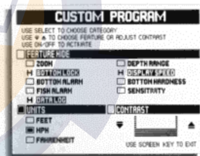
The SELECT button selects a function for adjustment The UP-DOWN buttons are used to select specific features or adjust contrast ON-OFF hides the selected function
